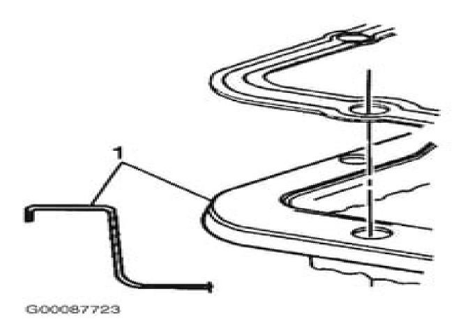
Fig. 5: Inspecting Oil Pan Flange Courtesy of GENERAL MOTORS CORP.
