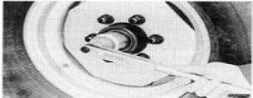
Rotate the wheel and tighten the nut to a torque of 100 Nm (74 lb ft), then back off the nut to the next slot.
