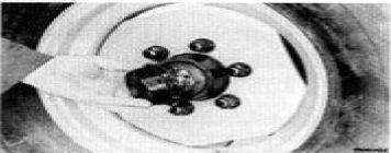
Install and tighten the dust cover.
