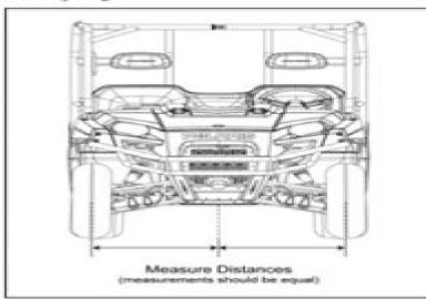
NOTE: Be sure steering wheel is straight ahead before determining which tie rod needs adjustment.
