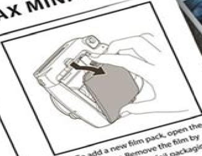
**STEP 2** To add a new film pack, open the back cover. Remove the film by opening the silver foil packaging.
