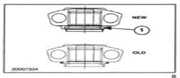
In order to install the new trunnion bearings on the wobble hub, you must install the seal ring, 2, on the wobble hub, 1.
