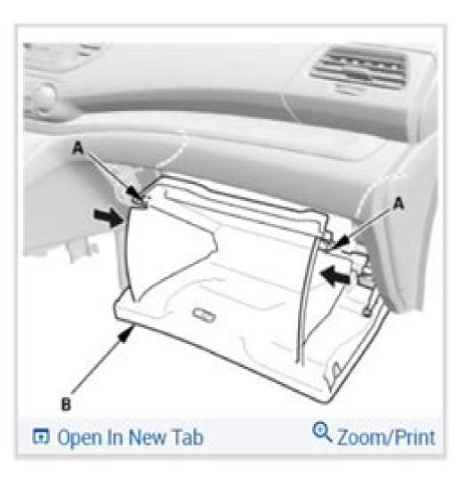
2. Release both glove box stops (A) by pushing them in, then let the glove box (B) hang down.
