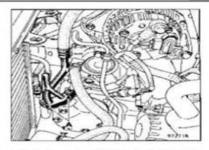
Remove the mounting bolt for the gearbox earth strap.
