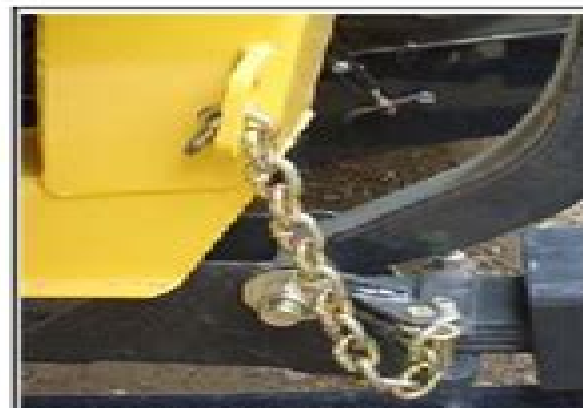
Loose Restrainer Chain
