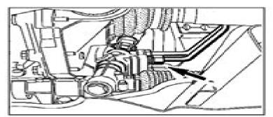
Drain the cooling circuit through the lower radiator hose.
