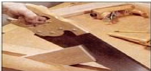
7 Use a crosscut saw to cut inclines on the top surface of the base members. Remove any cut marks by hand planing.
