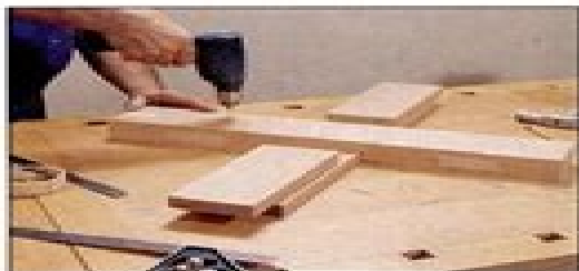
4 Dry assemble base components with masking tape and bore pilot holes for alignment nails that hold pieces square.
