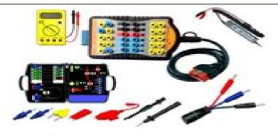
Switch testing tools where can plug any tester such as lab scopes, multimeter, logic probes, test lights etc.
