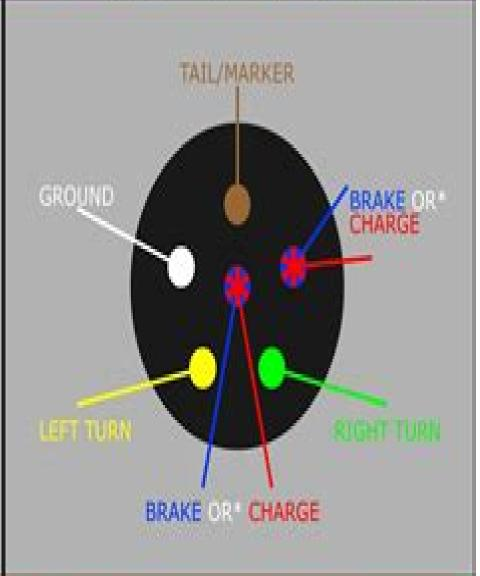
\*Brake and Auxiliary Power have two different industry standards. Identify which way your trailer is wired before wiring connectors.
