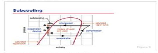
Inside the condenser, after all of the refrigerant vapor has condensed into liquid, the refrigerant is subcooled to further lower its temperature. This subcooled liquid refrigerant leaves the condenser (A) and experiences a pressure drop as it flows through the liquid line and accessories, such as a filter
