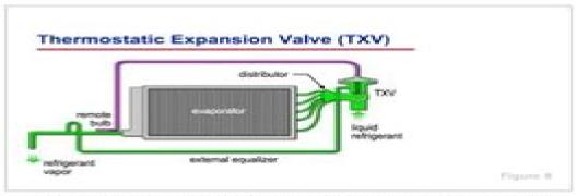
The second requirement of the refrigerant piping design is to ensure that only liquid refrigerant enters the expansion device. There are several types of expansion devices, including expansion valves (thermostatic or electronic), capillary tubes, and orifices.
