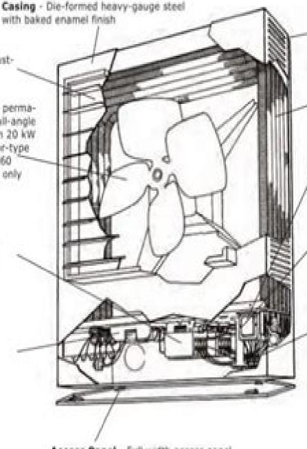
Access Panel - Full width access panel secured by quarter-turn fasteners.
