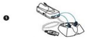
To install be so unit, first thread the USB sable through the bottom of the base on Ericula in the natch. Then attach the stand by inverting the stand pega into the holds on the underside of the base soil.
