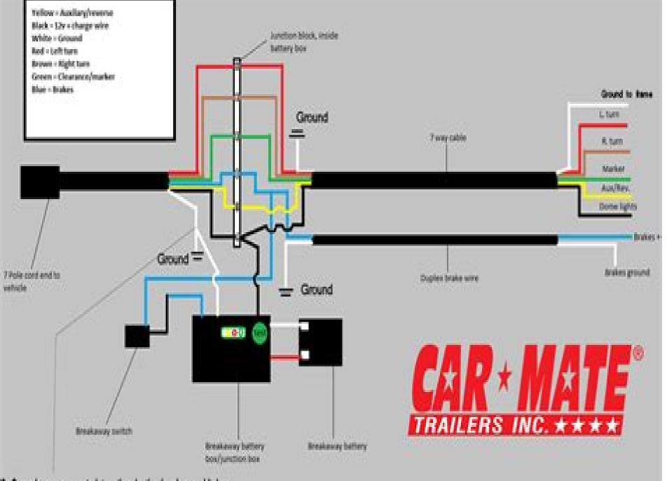
3 Grounds are connected together in the breakaway kit box
