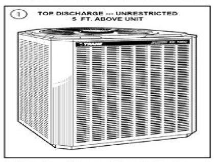
If the outdoor unit is mounted above the air handler, maximum lift should not exceed sixty (80) feet fauction lines. If air handler is mounted above the condensing unit, maximum lift should not exceed sixty (80) feet (liquid line).
