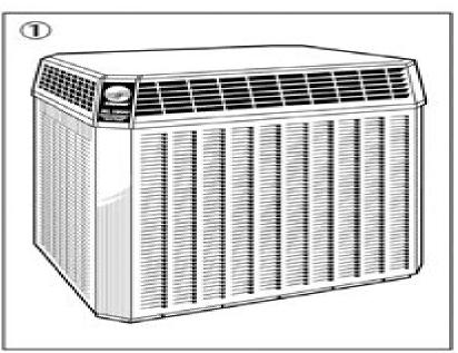
3. Avoid locating the unit where condensation and freezing of defrost vapor may annoy the customer. For instance, installing the unit under a bedroom, kitchen, or picture window may be annoying to the customer since condensate and fog will occur during the defrost cycle.
