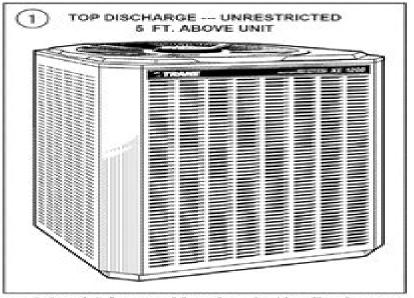
restriction of airflow to and from the unit. Also allow for proper maintenance space. The barrier should be constructed of materials which will blend in with the building design.
