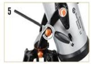
The altitude slow motion rod has a limited range of motion of about 15 degrees. If you run into the end of travel and the knob will no longer turn, you can reset it by loosening the rod guide knob and turning the slow motion rod handle the opposite direction until you are in the middle of its travel, then retighten the rod guide knob.
