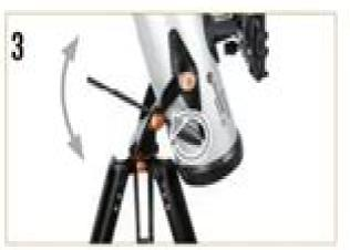
To move the telescope up and down, hold the focuser of the telescope in one hand and loosen the knob on the slow motion rod guide. The telescope can now be moved up or down as desired. When you are close to your target, tighten the knob to secure the telescope in place.
