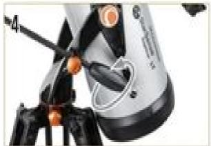
Fine adjustment in the up-and-down direction can be done using the altitude slow motion rod. Keep the rod guide knob locked and rotate the black handle on the slow motion rod. This allows you to move the telescope in small increments to help center objects or follow celestial objects in the night sky.
