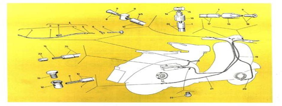
T. XVI Transmissions: Throttle - Clutch - Front brake
