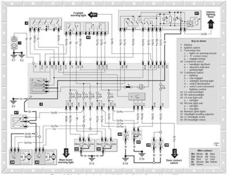
Diagram 6: Side, tail, number plate, head and loglights, headlight levelling - models up to 1998
