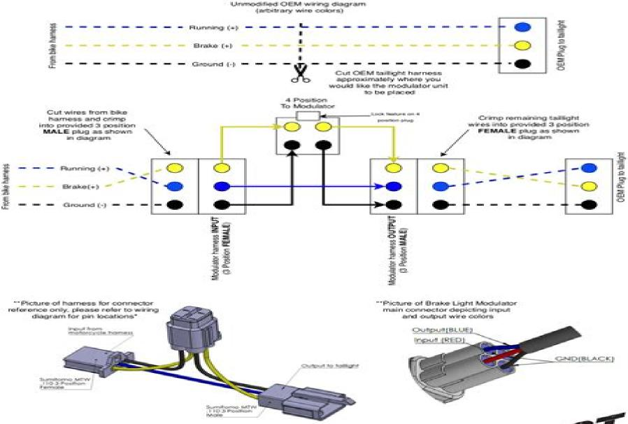
"Please note; since the running light signal (brown wire from bike) is not affected by the modulator, it is not necessary to cut and can be left out of the brake light modulator harness entirely if you so choose. If the brown running light wire is cut and crimped into the hamess, the blue wire will carry the signal through to the tailight leaving it unaffected by the modulator unit.
