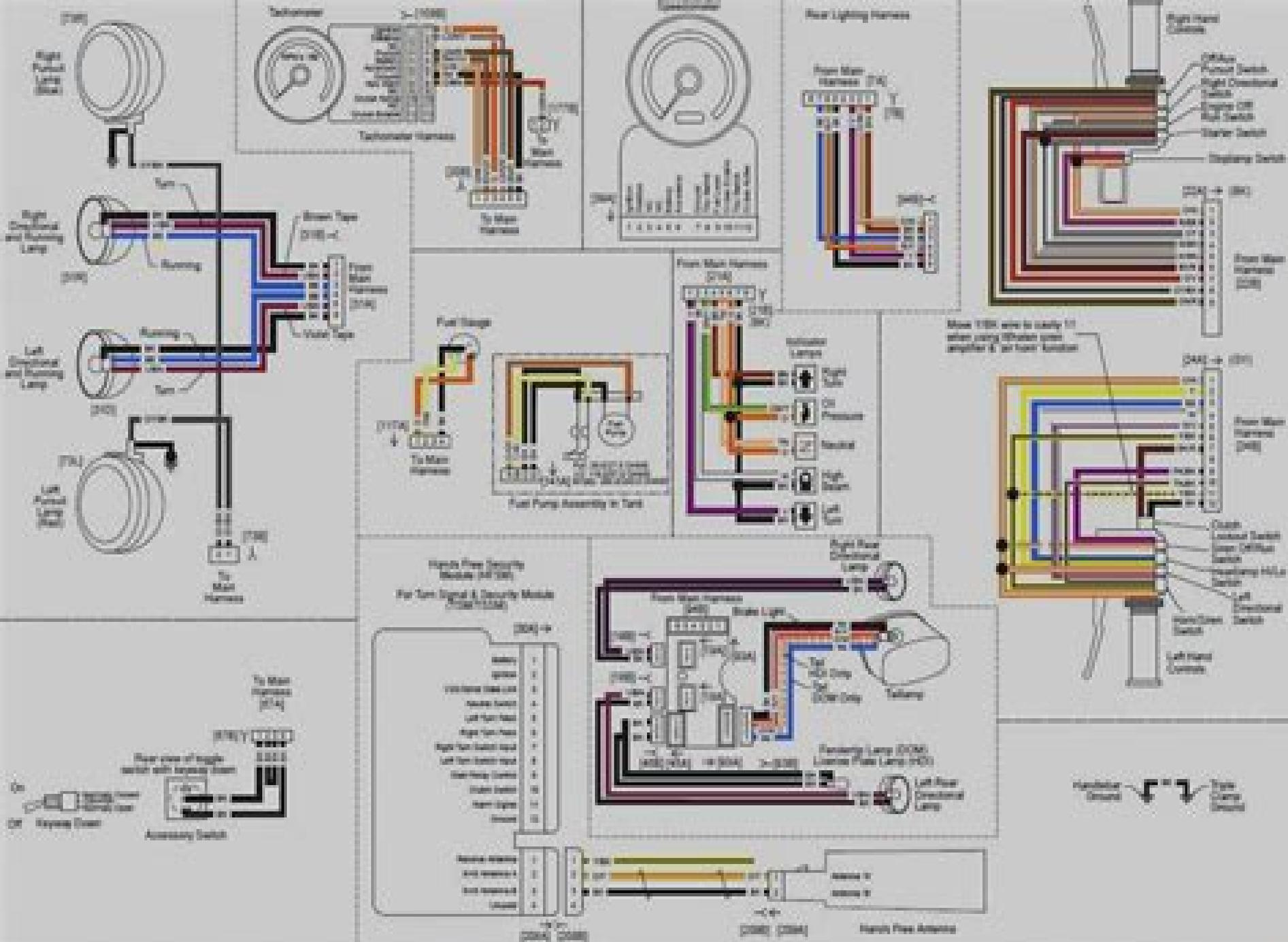
Figure A-15. Indicator Switches, Indicator Lamps, Tail Lamp, Parking Lamp, Directional Lamps, Accessory/Fuel Switch, Tachometer, and 12V DC Antenna. 1988 FIAT® and FIAT® DOMESTIC and INTERNATIONAL Models.
