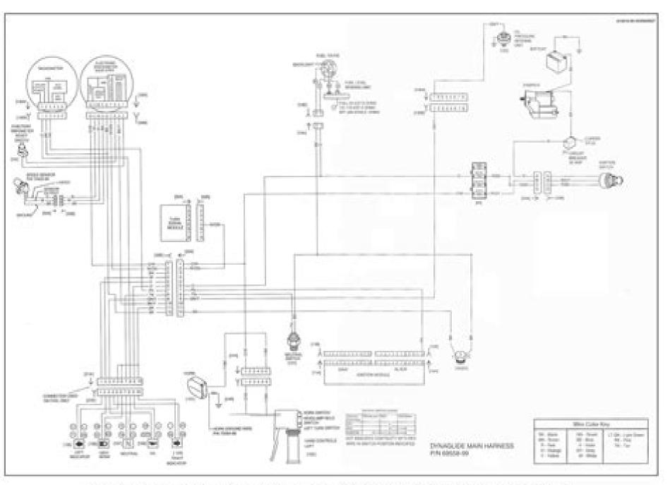
DYNA GLIDE WIRING DIAGRAM (Domestic and International Models), Horn and Instruments
