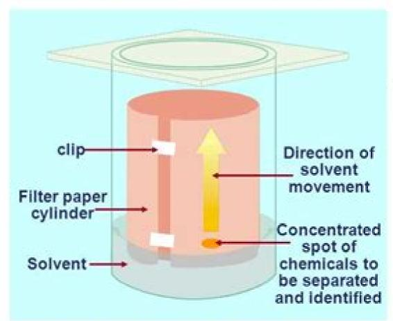
Paper chromatography is a technique used for the separation & identification of relatively small chemical substances by a moving solvent on sheets or strips of filter paper
