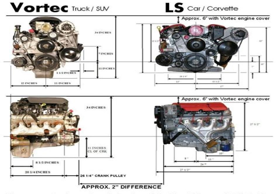
Oil pans can be changed easily to either style. The intake manifold height and accessory package depth is the biggest difference between Vortec & LS.
