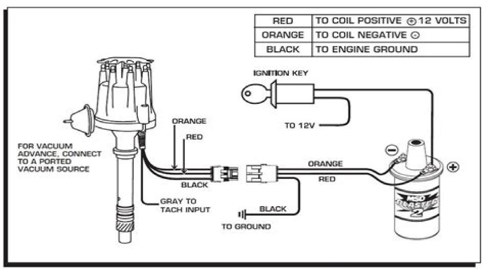
Figure 10 Wiring the Ready-to-Run Chevrolet Distributor.
