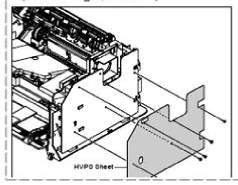
Separate the HVPS with HVPS frame by releasing the remainin (Screw x 3:Gold\_M3,6003-000)
