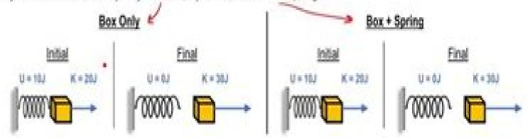
Mech. Energy in a system is CONSERVED if the ONLY forces doing work are \_\_\_\_\_ =
