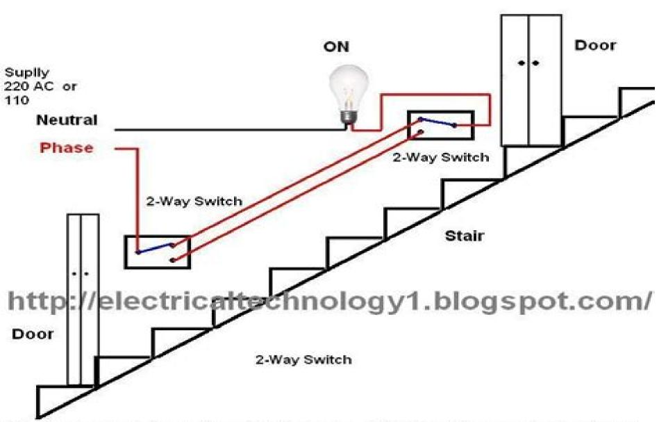
Stair case wiring circuit diagram, OR How to control a lamp from twoplaces by two ,2-way switches?
