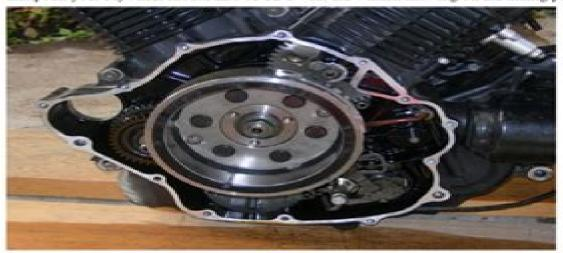
You can see in the photo above the Timing Marks. The Flywheel above is current set for TDC on Front Cylinder. Below is the inside of the Clutch Cover (Right Hand Side) and the cogs at the Front of the engine are the Crank and Camshaft Chain-Drive. They have Timing Indents which align after every 12 revolutions of the engine... once they are aligned your front cylinder is definately at TDC and you can then set your Cam Timing accordingly.
