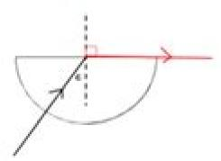
The angle of incidence in this case is called the critical angle (c) of the material.
