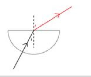
If the angle of incidence is exactly right, however, this will give an angle of refraction of exactly 90°:
