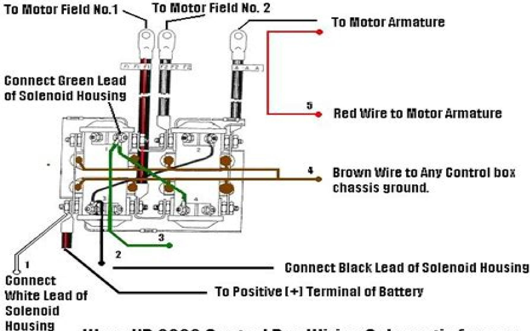
**Warn XD 9000 Control Box Wiring Schematic for use
