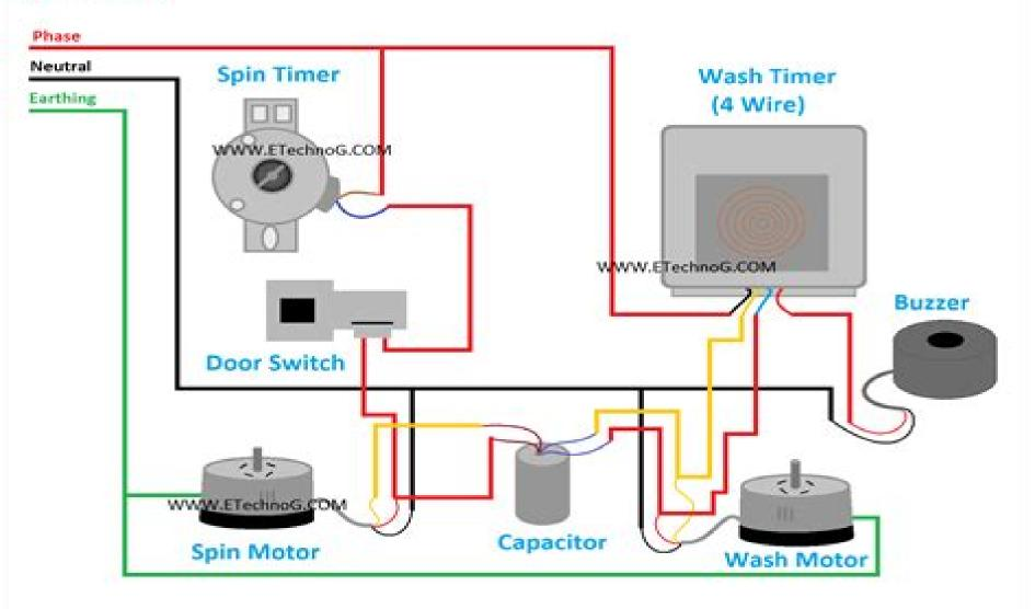
Washing Machine Wiring and Connection Diagram
