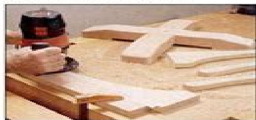
10 Ease sharp edges using router with rounding-over bit. Hold small pieces to a clamped scrap piece with masking tape.
