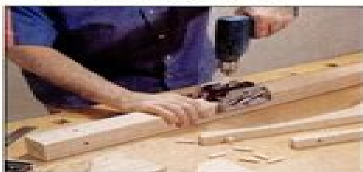
11 Bore dowel holes in post and post supports using a doweling jig. Attach tape to drill bit to act as depth gauge.
