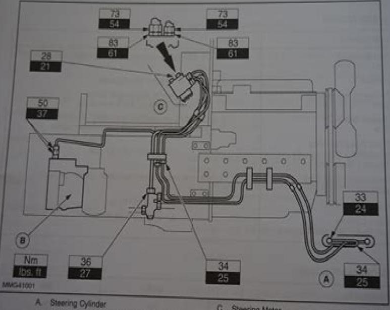
Variable Displacement/Tandem Gear Pump
