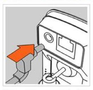
Connect the power adapter to the power jack on the back of the camera and plug the other end into the power outlet.
