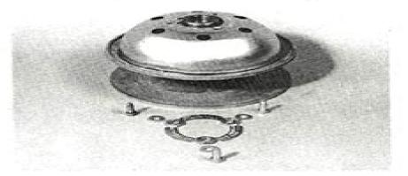
Remove the snap ring, using a snap ring pliers. NOTE: Fixed face shaft has two (2) grooves for snap ring installation; observe which groove snap ring occupied and install in the same groove when reassembling.
