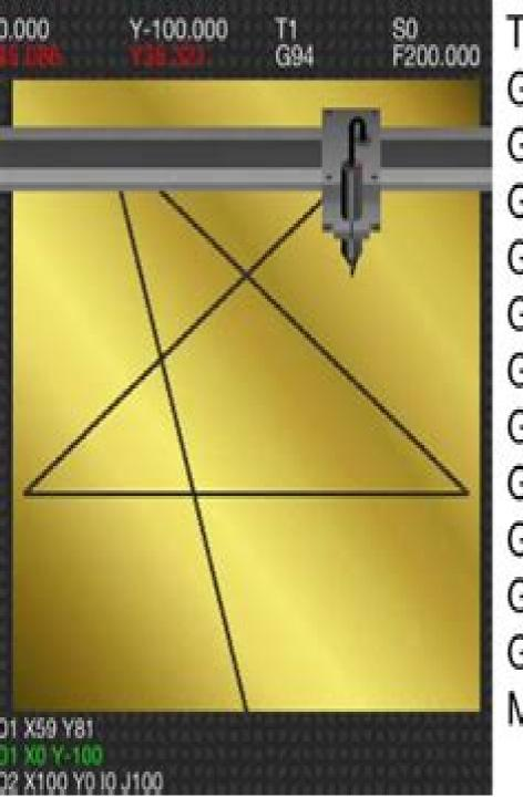
T1 M6 G90 G94 G54 X0 Y0 G00 X0 Y0 G00 X0 Y-100 G01 X-59 Y81 F200 M3 G01 X95 Y-31 G01 X-95 Y-31 G01 X59 Y81 G01 X0 Y-100 G02 X100 Y0 I0 J100 G02 X0 Y-100 I-100 J0 M30;
