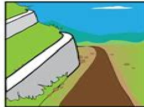
An area in South Carolina has had mudslides. The community has installed a retaining wall. This will help to hold water-saturated soil in place and prevent mud from spilling onto the road.
