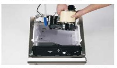
Remove four 5/32" allen head screws holding adapter to evaporator
