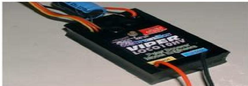
The VIPER ESC's do not have directional constant brightness lightness output controls. Use the RCS # **REV-LT** to have automatic constant brightness directional lighting.
