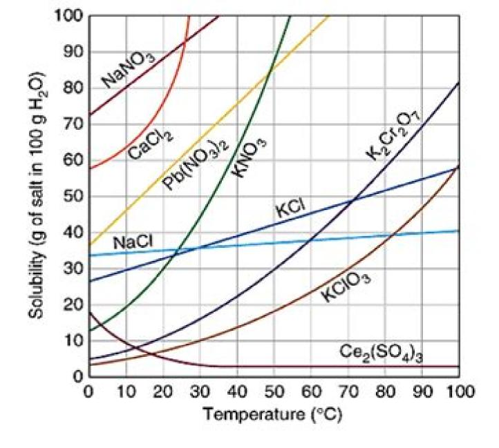
Figure 1. Solubility curves for several ionic solids in H<sub>2</sub>O.
