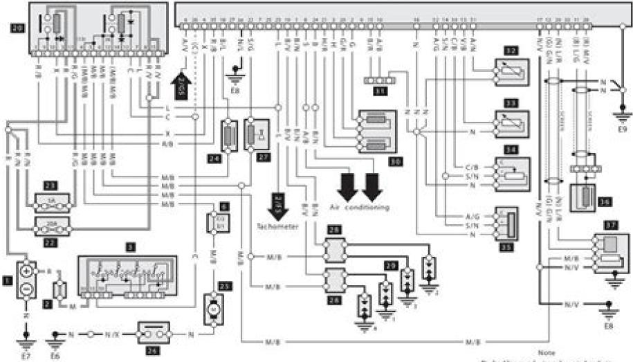
Disched lines and wire colours in brackets denote variation for single point wiring.
