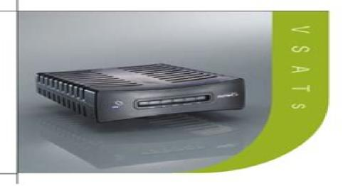
Inbound efficiency is maximized with 8PSK support and DVB-RCS based turbo coding. The VSAT uses ICM technology on the inbound that provides 3 dimensions of adaptivity: tx power, ModCod (coding and modulation) and symbol rate. These combine to ensure high availability with a maximum dynamic range of up to 23dB.
