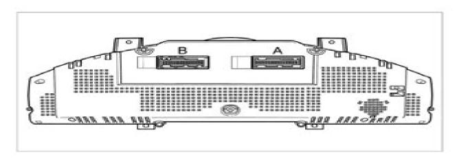
Wiring harness plug A, 32-pin instrument cluster/gateway
