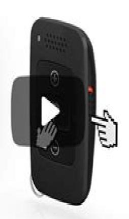
Hold down the "P" button on the remote control while switching the key lock to the unlock position.
