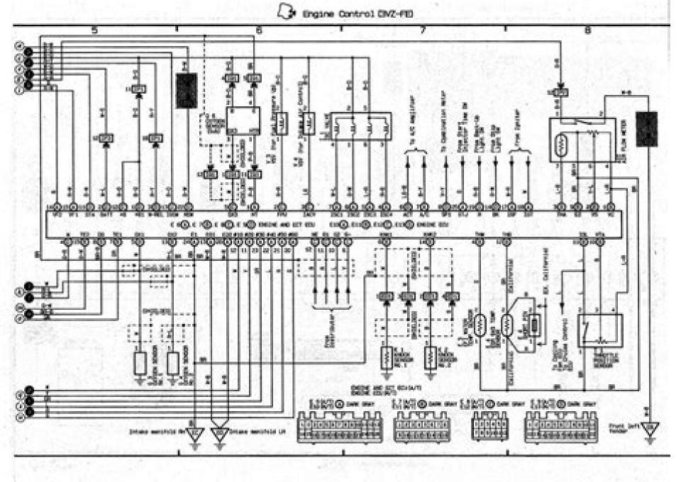
Typical 3VZ-FE V6 engine control system wiring diagram (1963 and earlier models) (2 of 2)
