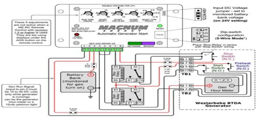
Relays used are SPDT 30 Amp, 12 VDC coil relays [shown in the non-energized (N.C.) position]; popular in automotive sound and security installations. Equivalent to Bosch #0 332 209 150. Mfg. #V23234-A1001-X036.
